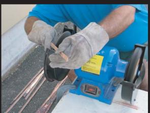
2) I then strip, burn, clean, scrape, brush, straighten... in other words, this step is the most labor intensive part of the process. Once prepped, I end up with gleaming, straight pieces of metal that will be used in the following step.
